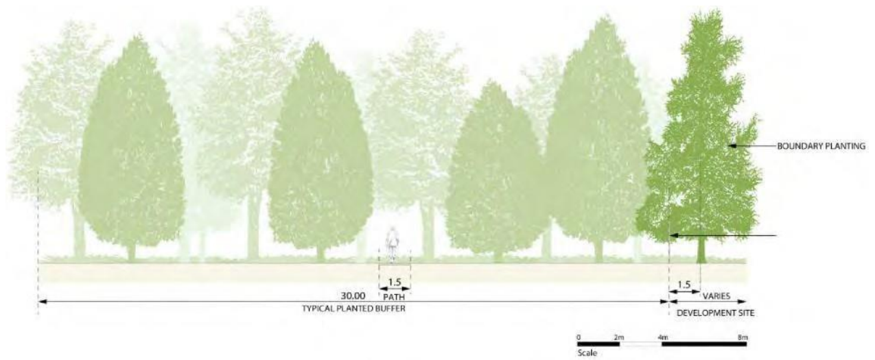
Diagram 5: Typical landscape buffer cross section
