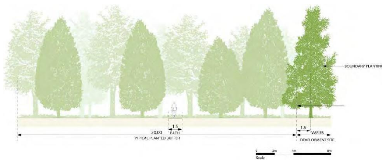
Diagram 5: Typical landscape buffer cross section
