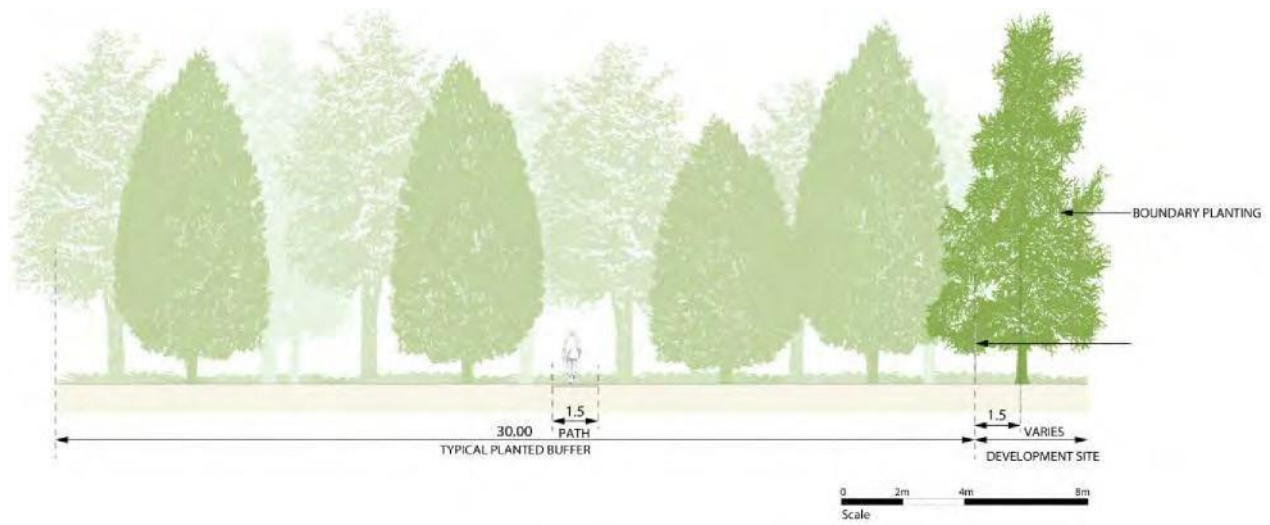
Diagram 5: Typical landscape buffer cross section
